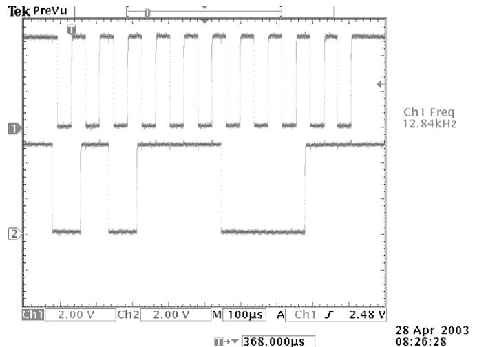
Note also that when you depress a key, the keyboard issues two codes in sequence: x"F0" followed immediately by the key's scan-code. Since we display the codes on the LEDs when they arrive (without extra delay), you will probably miss the F0 and only observe the scan code.
