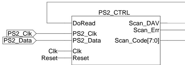
**Reset** is used inside the module as an asynchronous and global reset.
